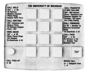
Plate Mounted over the Dial of the Telephones at the University of Michigan. These inadequate instructions are all that most users see. (The button labeled "TAP" at the lower right is used to transfer or pick up calls—it is pressed whenever the instruction plate says "TAP." The light on the lower left comes on whenever the telephone rings.)
